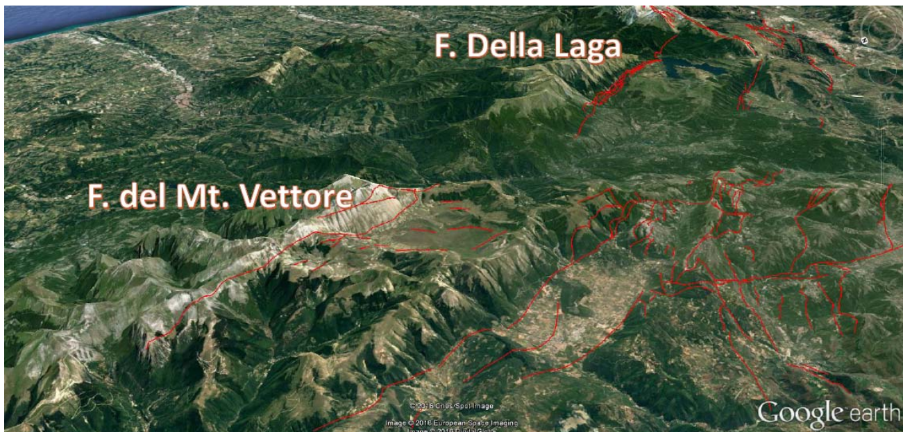
Fig. 3 – Capable faults in the epicentral and surrounding areas, according to ITHACA (source: ISPRA). View from northwest.
