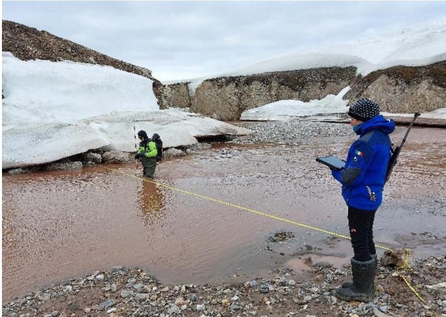
Flowrate measurement on the Bayelva River (from left to right, Marco Doveri and Ilaria Baneschi (IGG-CNR)).
